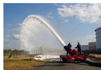
High-capacity foam water canon (Oita Refinery)
